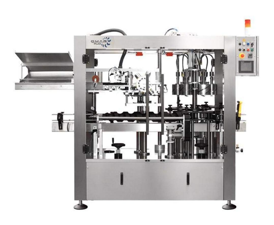
Machines for the distribution and closure of PVC, aluminium, polylaminate and tinfoil capsules with single or multi-cup dispensers, shrink heads and spinning heads with speed rates from 1,000 to 8,000 b/h.
