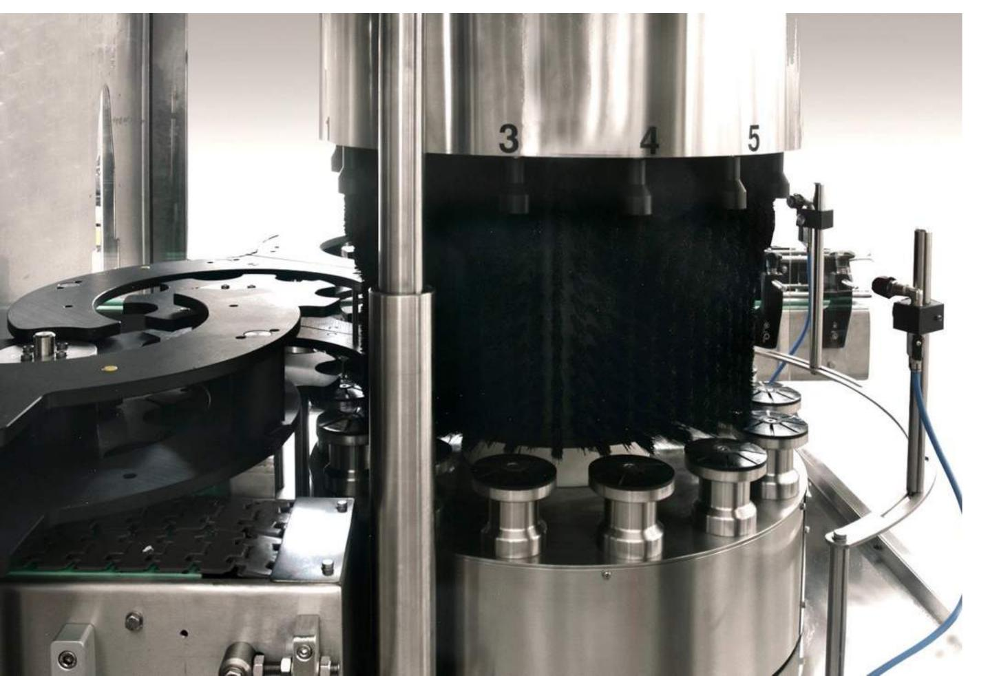
Machines suitable for the washing and drying of cylindrical and shaped bottles with speed rates from 1,000 b/h to 20,000 b/h.
