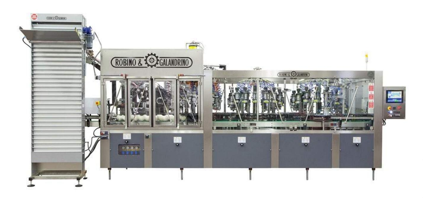
Distributor and capsuling monoblock comprised of a frame manufactured of electrowelded steel and covered by stainless steel.
