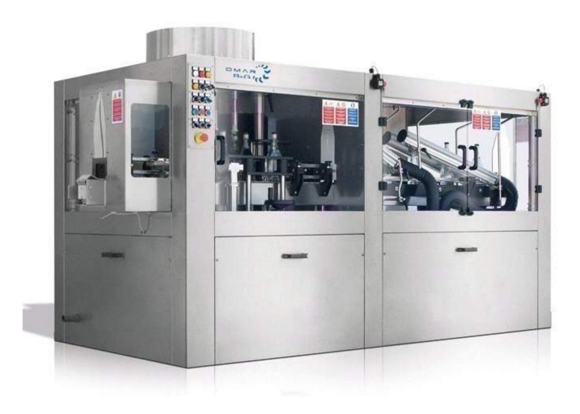
Machines suitable for the washing and drying of cylindrical and shaped bottles with speed rates from 1,000 b/h to 20,000 b/h.
