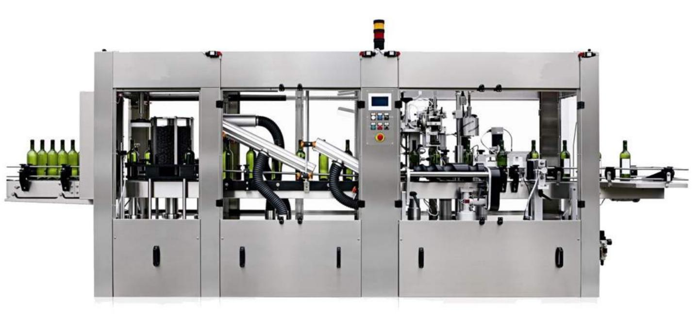
The monoblocks of the SYMPHONY series bring together, in a single solution, all the stages of wine packaging for the most demanding of producers: washing, drying, capsuling and labelling.
