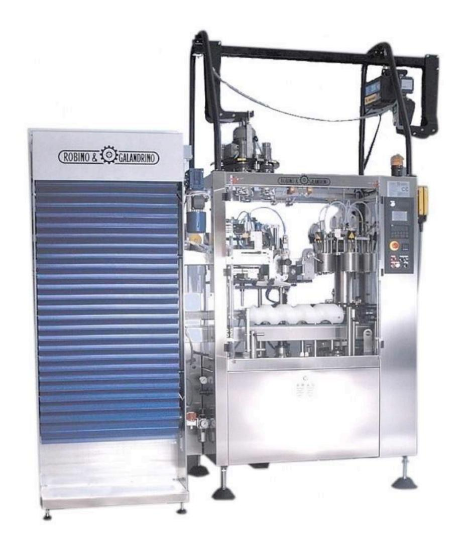
The dispensing and spinning monobloc type Superbloc is a compact capsule application machine complete with:
